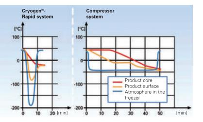
Cryogenic nitrogen or carbon dioxide not only achieve this very effectively, they do so economically as well. In Messer's cryogenic freezing applications named Cryogen®-Rapid the goods to be frozen come into direct contact with the refrigerant.
